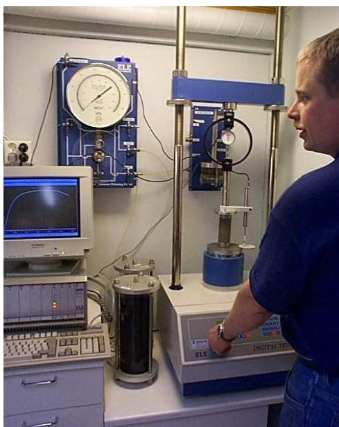
Figure 1. Unconfined compressive test in progress. Ramboll Finland Oy.
