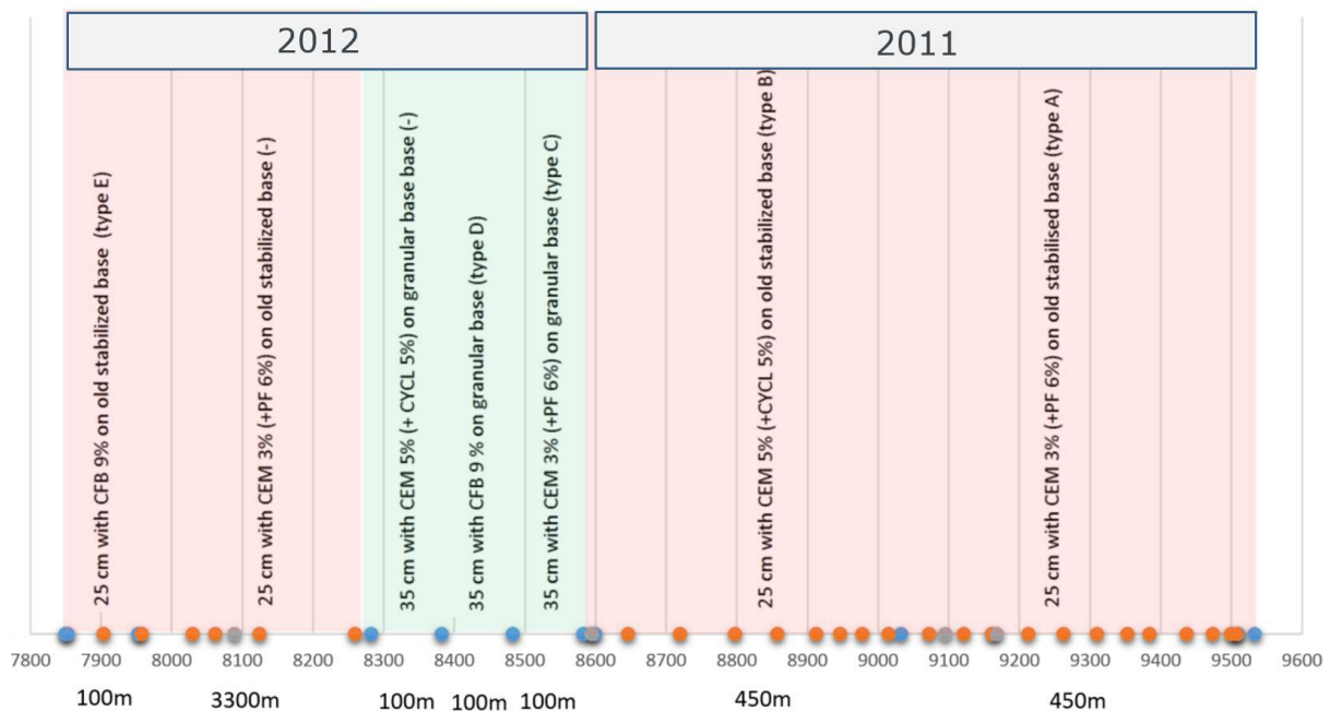
Figure 7. Location of cracks 2015 (orange dots).
