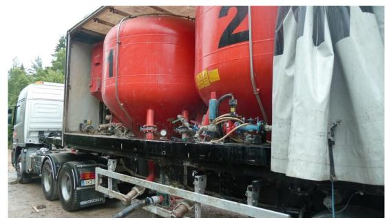
Photo 4-3 Binder material tanks (OSA and cement)
