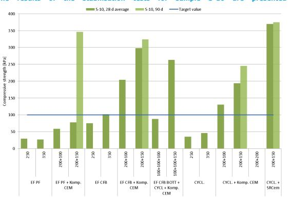
The results of the stabilisation sample **S-10** presented in tests for are
