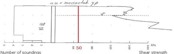
Figure 5-3 The average shear strength of stabilised peat in block 3VPL-4. The age of mass stabilisation is 87 days. Used binder material mixture is BL3 + KS (180 + 100 kg/m<sup>3</sup>).
