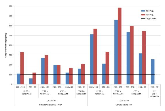
**Figure 3-9 Results of the stabilisation tests for Simuna-Vaiatu PR -samples, two lower layers.**
