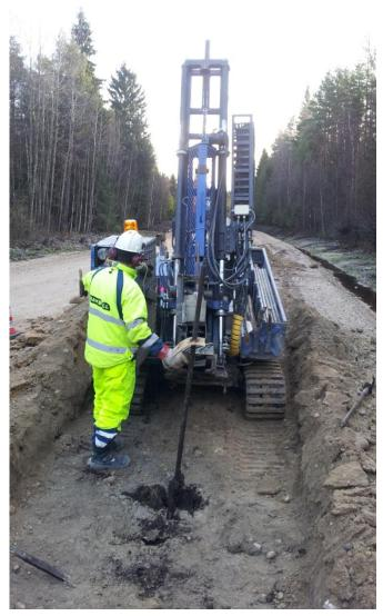
Photo 5-3 Cone penetration and vane share tests ongoing
