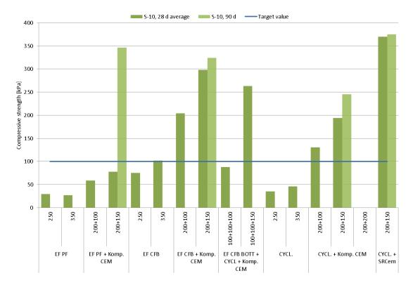
Figure 3-7 Results of stabilisation tests for sample S-10
