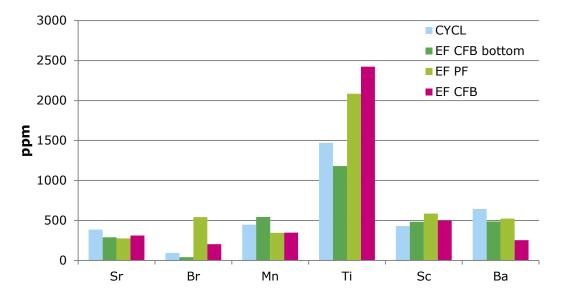
Figure 3-3 can be seen in titanium concentration. Electric filter ashes have the biggest titanium concentrations and the bottom ash has the smallest. EF PF has also the biggest bromine concentration. EF CFB had lower barium concentration than the other ashes.
