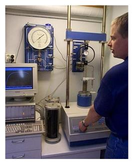
Photo 3-1 Unconfined compressive test in progress.
