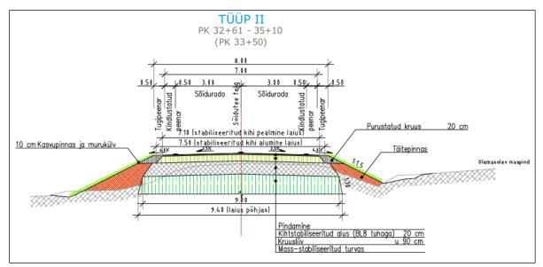
Figure 3-10 Road cross section and pavement structures
