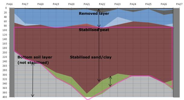
Figure 4-3 The layers of the removed material, peat, sand/clay and bottom soil. The depth is represented on left axis and the sampling points are represented on the top axis.
