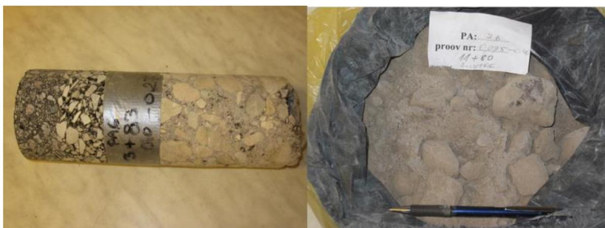
**Figure 6-1. Example of piece: sample 6, and loose: sample 26**
