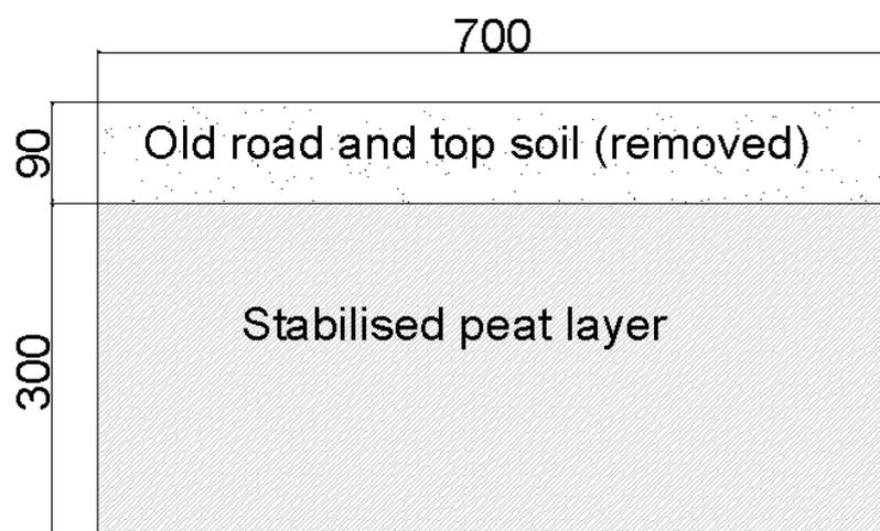
**Figure 4-2 The cross cut of the road – old road and top soil removed and the stabilised peat layer.**
