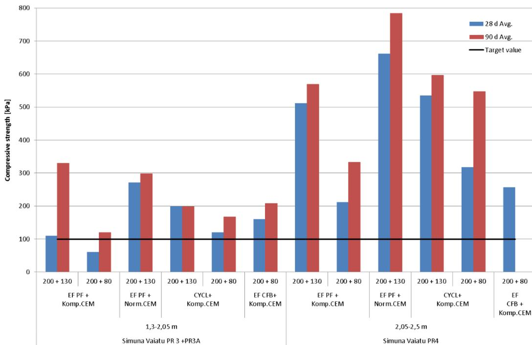
Figure 3-9 Results of the stabilisation tests for Simuna-Vaiatu PR -samples, two lower layers.
