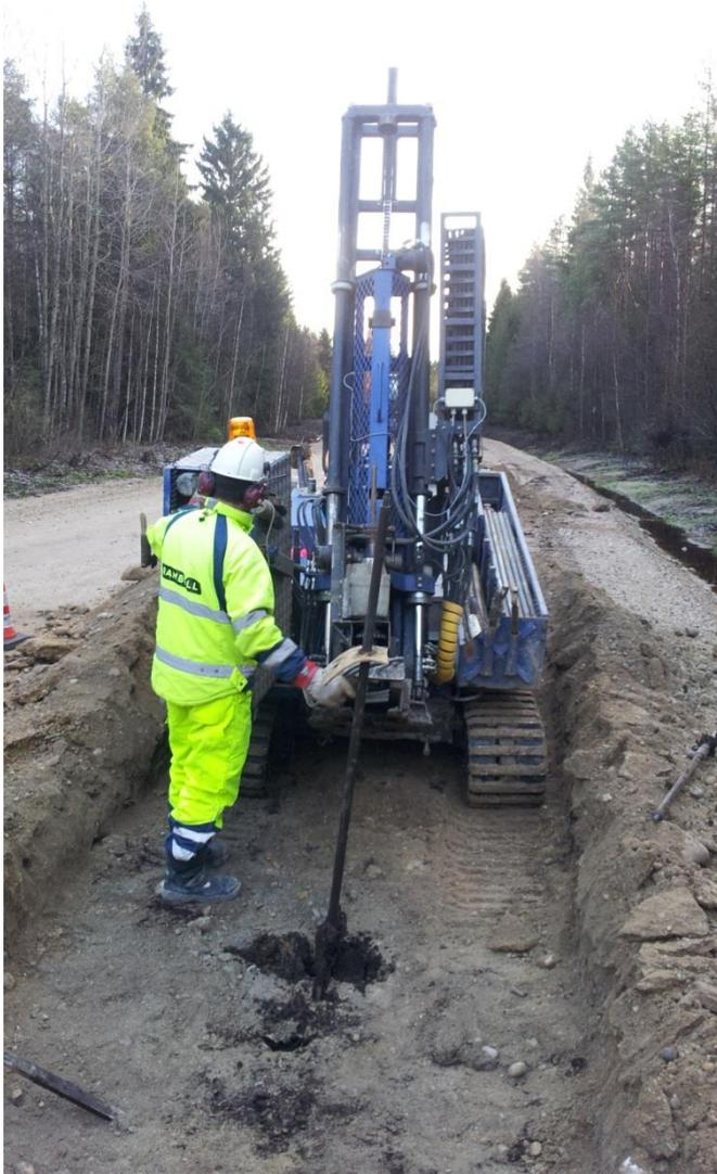
**Photo 5-3 Cone penetration and vane share tests ongoing**
