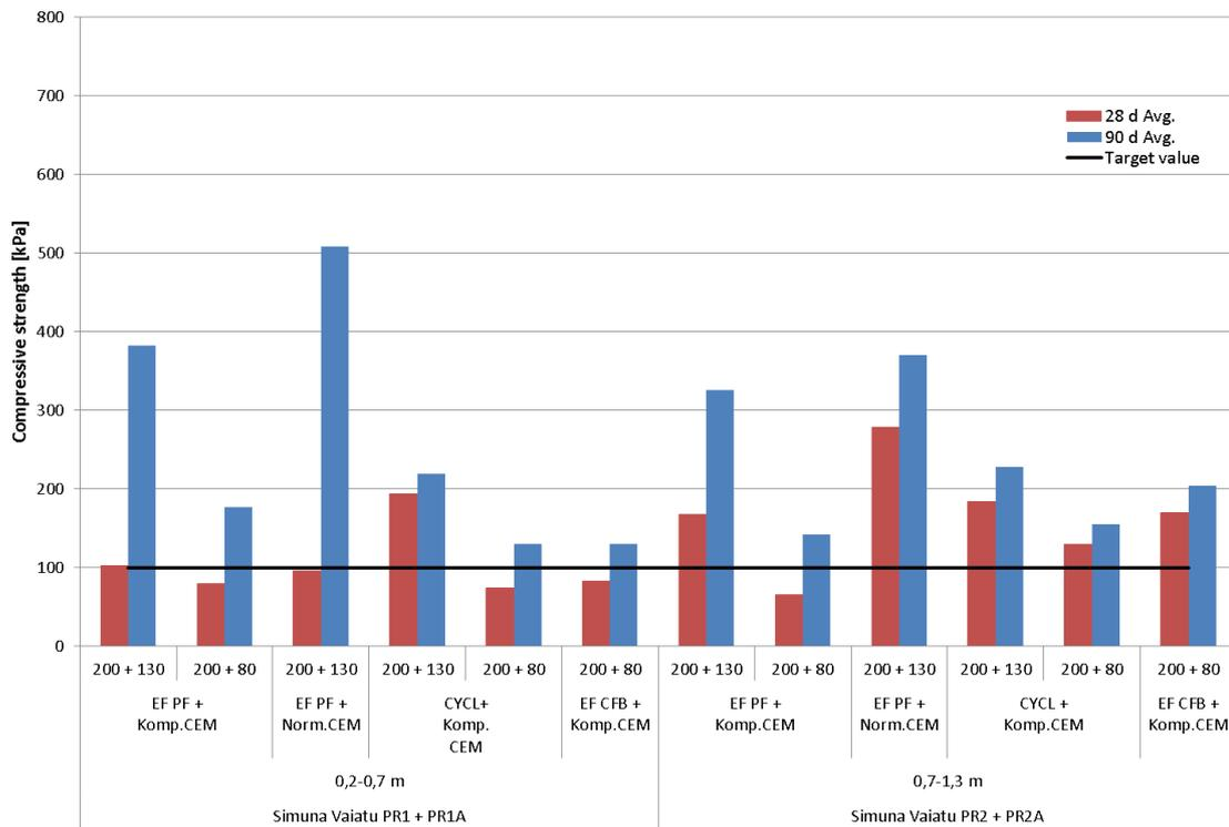
Figure 3-8 Results of the stabilisation tests for Simuna-Vaiatu PR -samples, two most upper layers.
