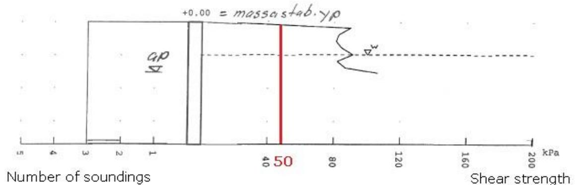
**Figure 5-2** The average shear strength of stabilised peat in block 16PPL-1. The age of mass stabilisation is 122 days. Used binder material mixture is CYCL + KS (200 + 60 kg/m<sup>3</sup>).
