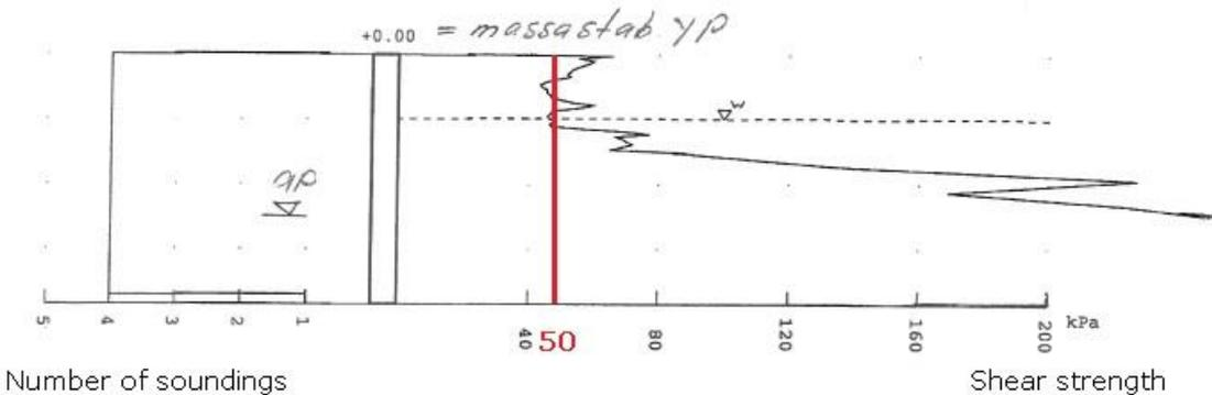
**Figure 5-1** The average shear strength of stabilised peat in block 11VPL-2. The age of mass stabilisation is 104 days. Used binder material mixture is EF PF + KS (190 + 90 kg/m<sup>3</sup>).
