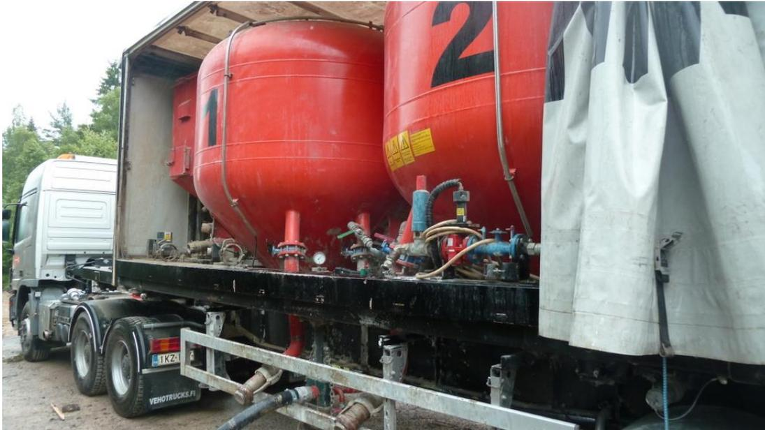
**Photo 4-3 Binder material tanks (OSA and cement)**
