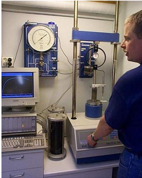
Photo 3-1 Unconfined compressive test in progress.
