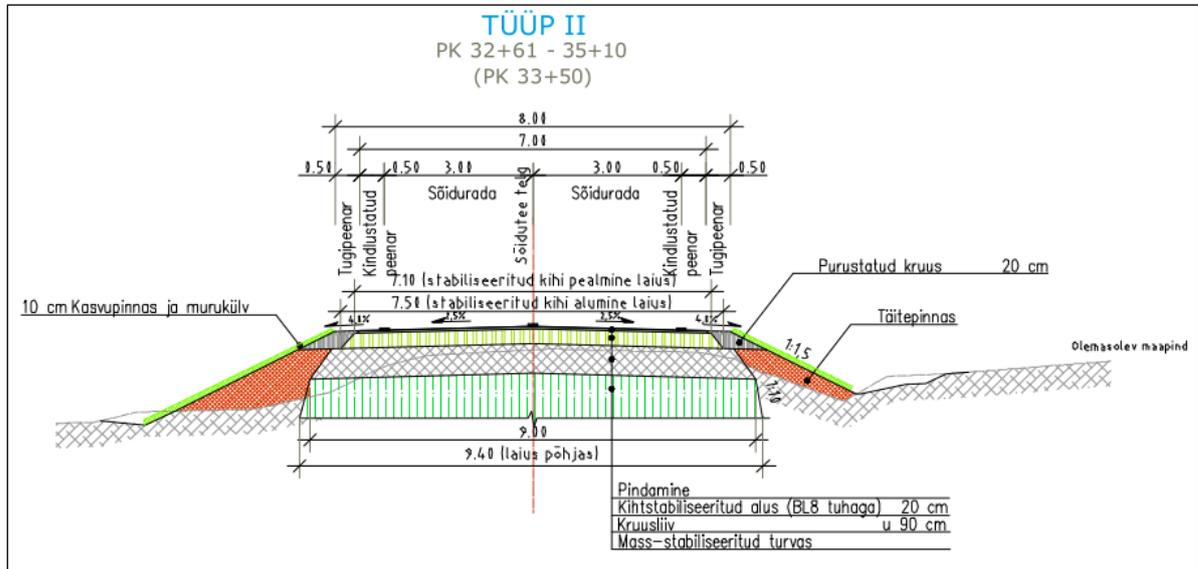
Figure 3-10 Road cross section and pavement structures
