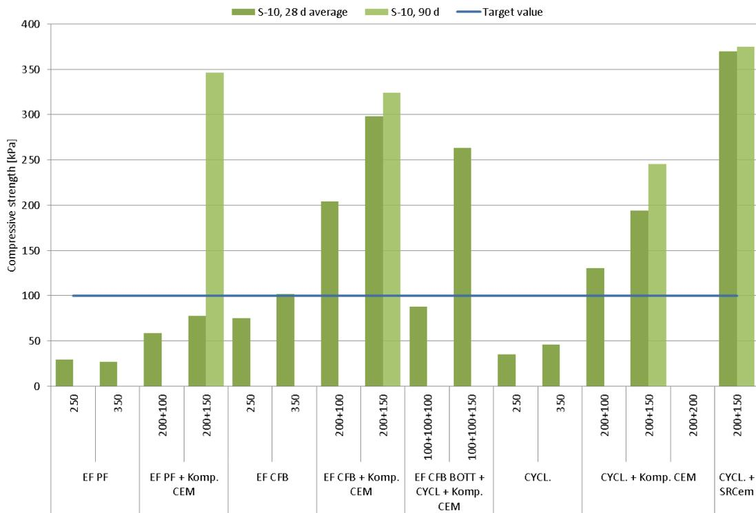
Figure 3-7 Results of stabilisation tests for sample S-10
