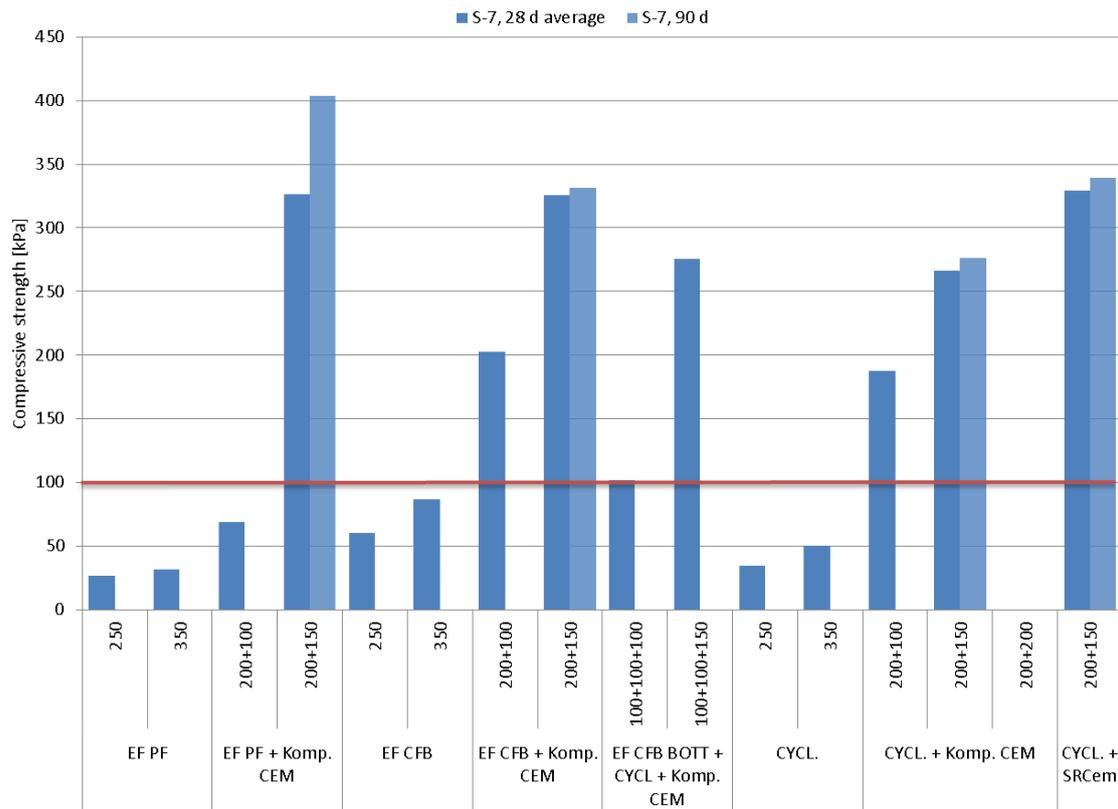
**Figure 3-5 Results of stabilisation tests for sample S-7**
