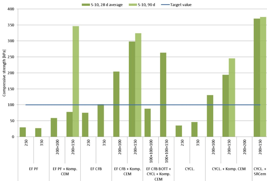
Figure 3-7. The sample S-10 gives similar compressive strengths compared with S-7. The difference between the 28 d and 90 d compressive strengths are small in all the other binder mixtures, but EF PF + Composite Cement, which has over 250 kPa difference between the 28 d and 90 d samples. All the peat samples achieved the targeted 100 kPa compressive strength.
