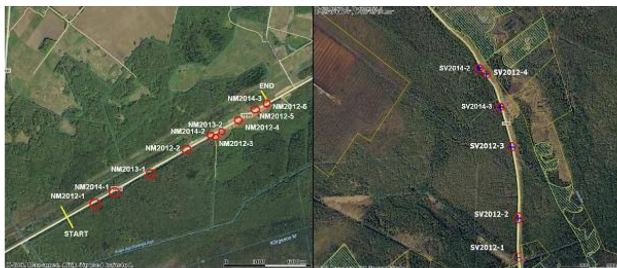
Figure 4. Soil sampling points in previous and current monitoring programs in Narva-Mustajõe (left) and Simuna-Vaiatu (right) pilot sections.
