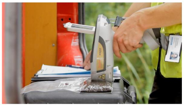
Figure 1.1. On site measurements with the Niton XL3t device.
