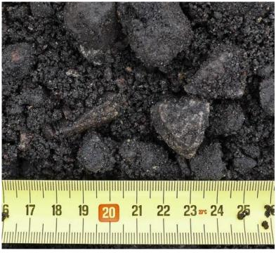
Figure 3-8. Milled and crushed asphalt concrete (MAC)
