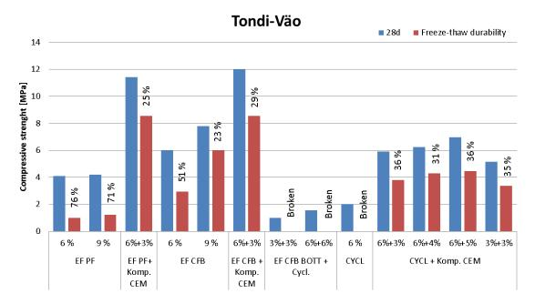
Figure 3-2. Stabilisation test results for Tondi-Väo aggregate
