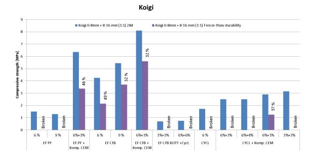
Figure 3-3. Stabilisation test results for Koigi aggregate
