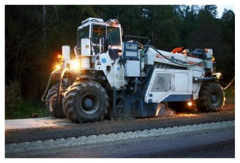
Figure 4-6. The Rotary mixer used in stabilisation work
