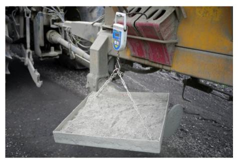
Figure 4-10. Binding agent spread measurement during spreading
