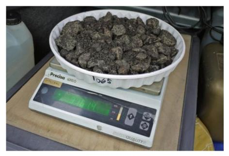
Figure 4-2. Dried body material weighed for water content analyses
