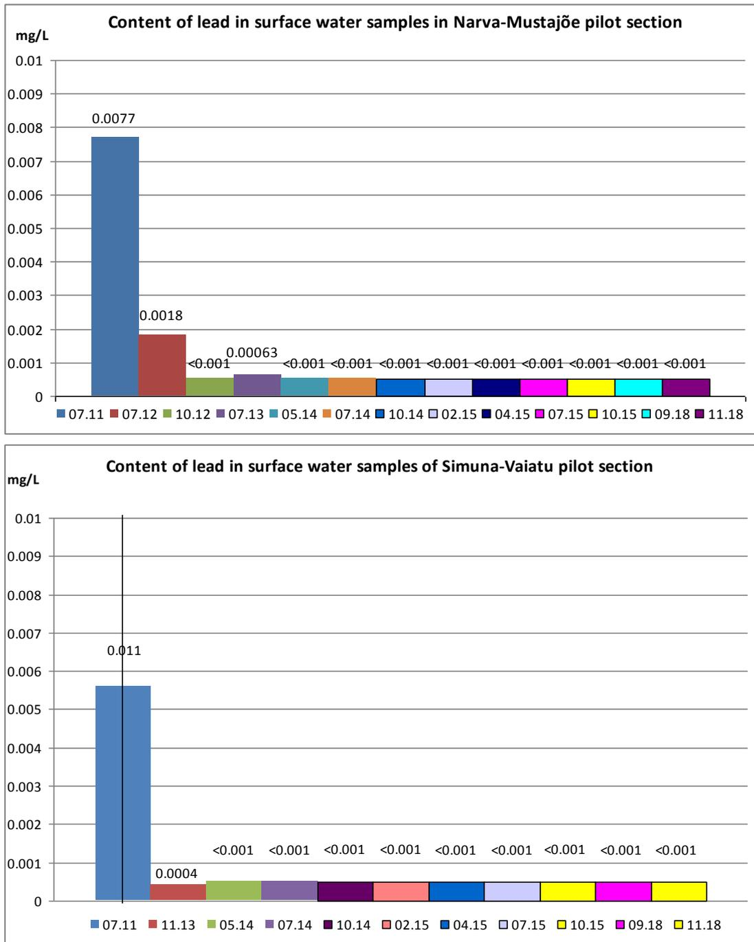
Figure 13. Observed content of lead in water samples of Narva-Mustajõe and Simuna-Vaiatu pilot sections (MAC-ECS for lead in surface water is 0.014 mg/L, 07.11 analysis from non-filtrated sample).
