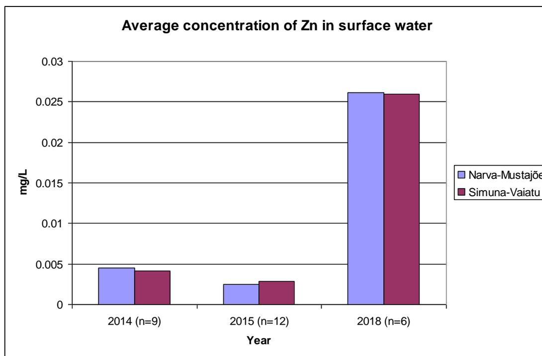
Figure 18. Average concentration of zinc in surface water samples during follow-up monitoring- values below LOQs are halved.
