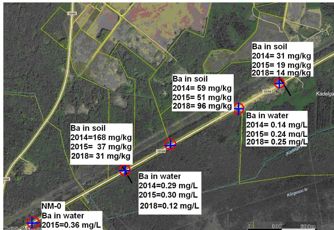
Figure 17. Barium content in soil samples and annual average barium content in surface water samples (except for NM-0).
