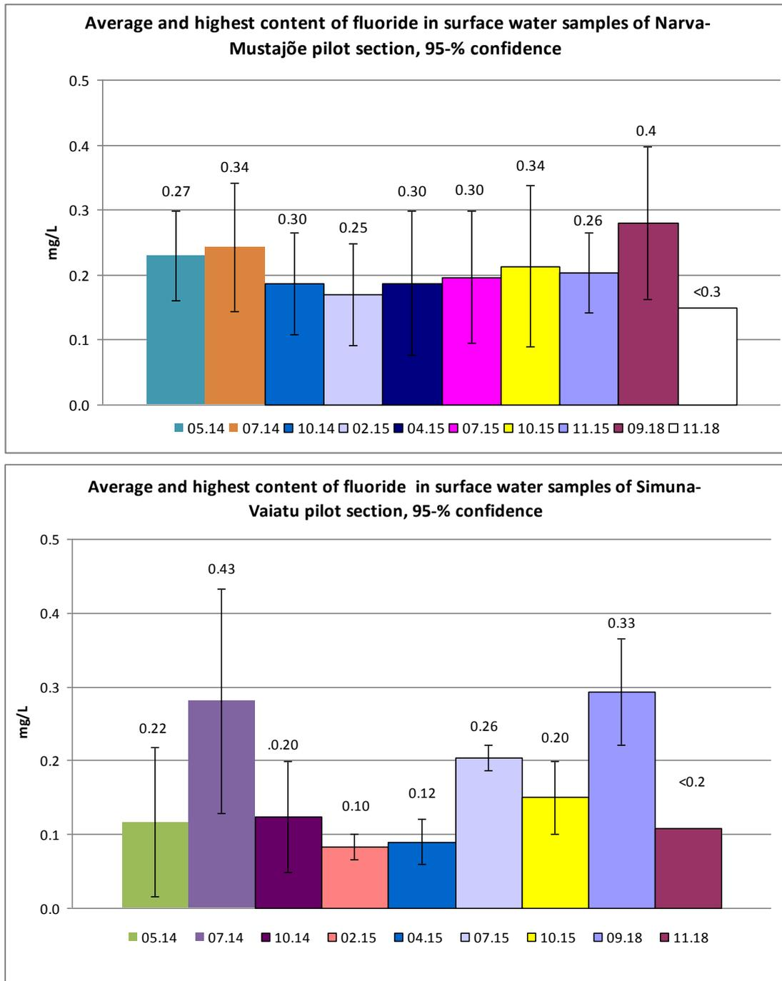
Figure12. Observed content of fluoride in water samples of Narva-Mustajõe and Simuna-Vaiatu pilot sections (Limit concentration 1.5 mg/L).
