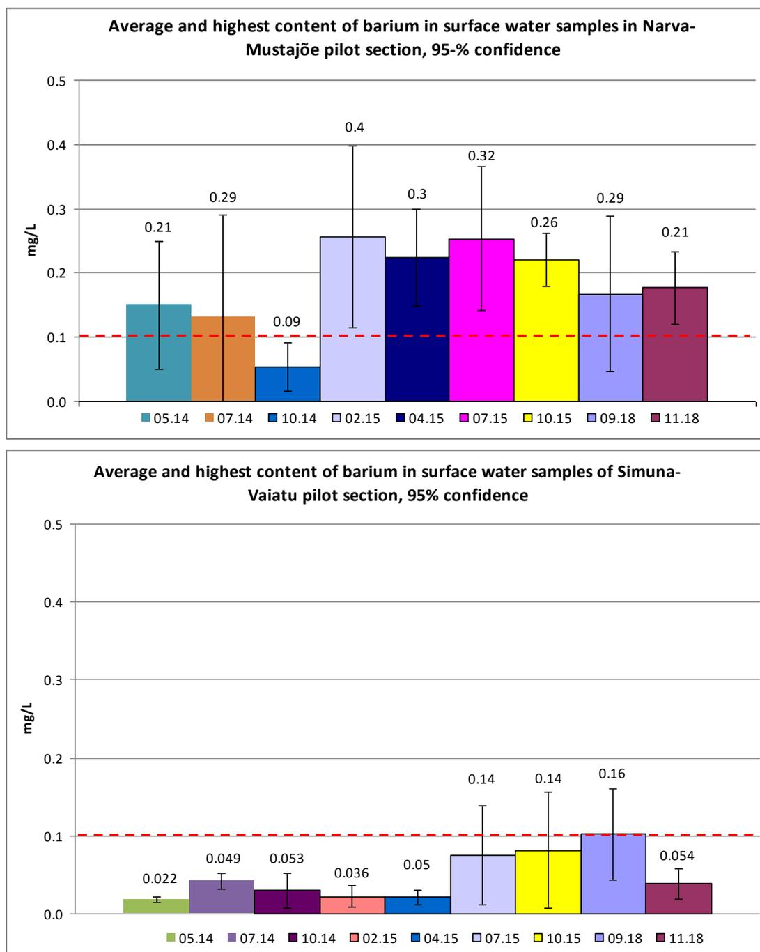
Figure 16. Observed content of barium in water samples of Narva-Mustajõe and Simuna-Vaiatu pilot sections (MAC-EQS for barium in surface water is 0.1 mg/L).
