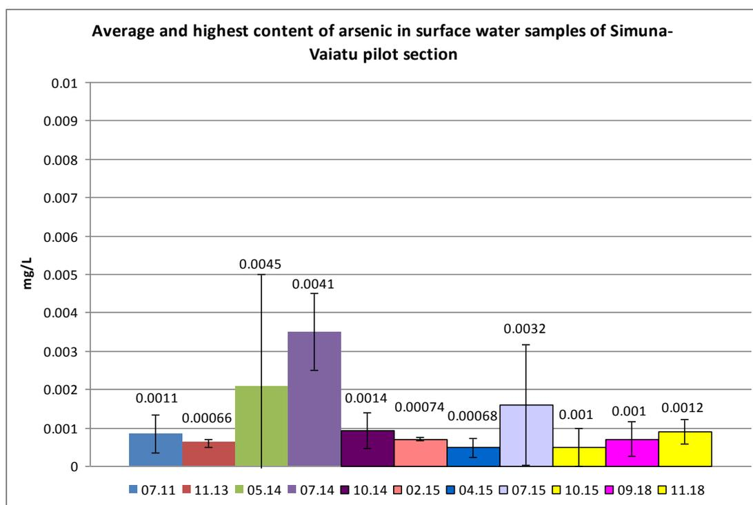
Figure 14 Observed content of arsenic in water samples of Narva-Mustajõe and Simuna-Vaiatu pilot sections (MAC-ECS for arsenic in surface water is 0.01 mg/L, 07.11 analysis from non-filtrated sample).
