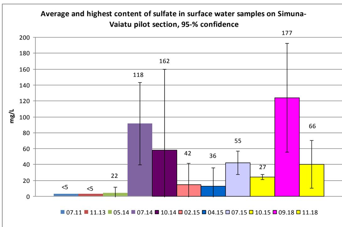
Figure 11 Observed content of sulfate in water samples of Narva-Mustajõe and Simuna-Vaiatu pilot sections. NB! Different scales.
