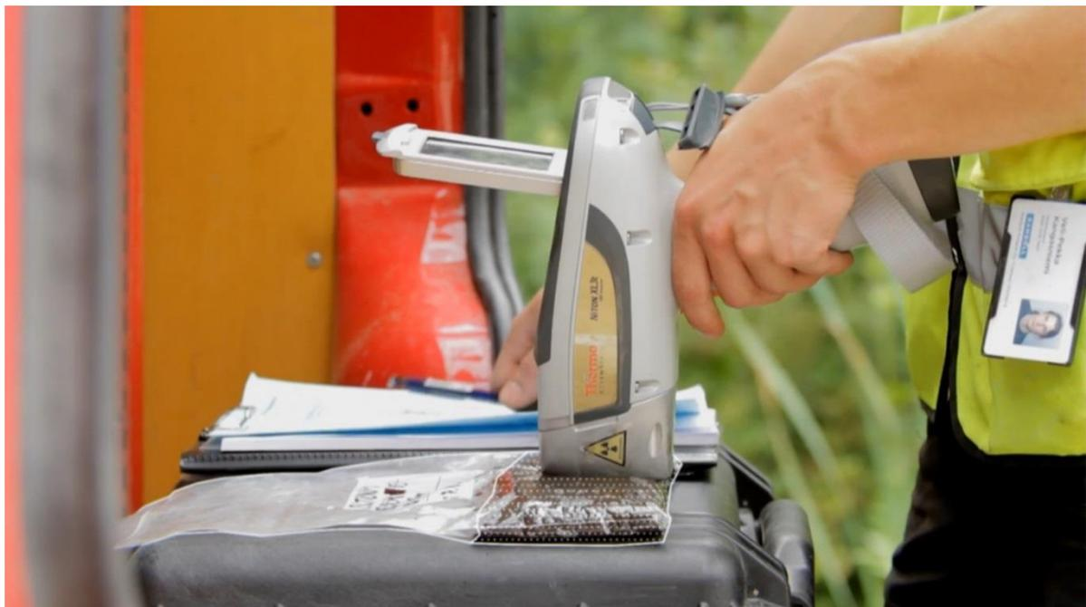
**Figure 1.1. On site measurements with the Niton XL3t device.**
