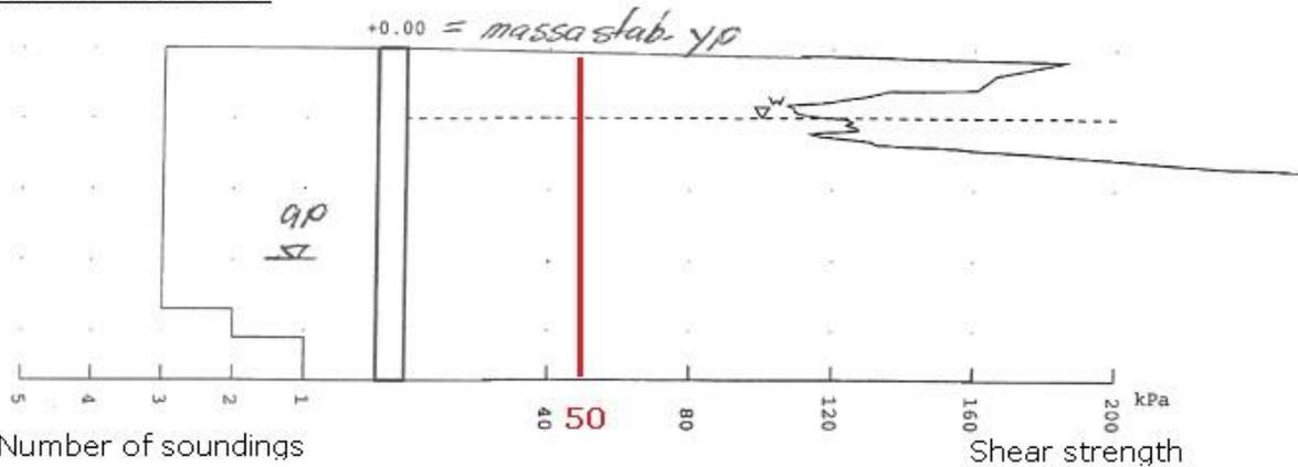
**Figure 1.7a. The average shear strength of the stabilised peat in block 19 PPL-4. The age of the mass stabilisation is 120 days. Used binder material mixture is EF PF + KS 180 + 100 kg/m<sup>3</sup>.**
