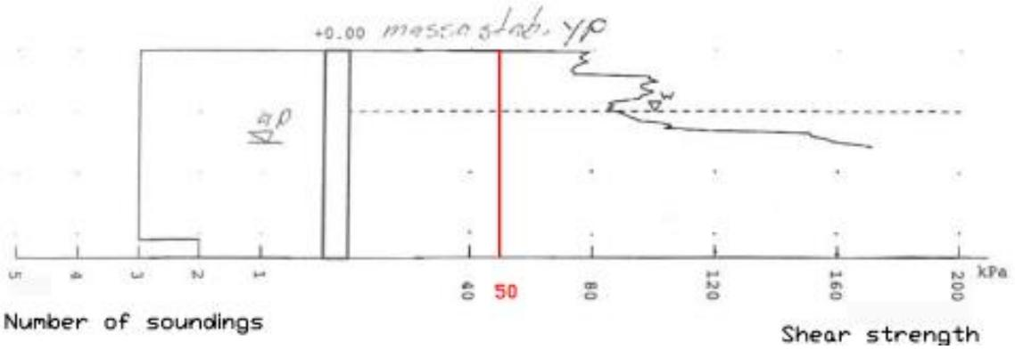
**Figure 1.3b.** The average shear strength in block 15 PPL-1 at the age of ten months.
