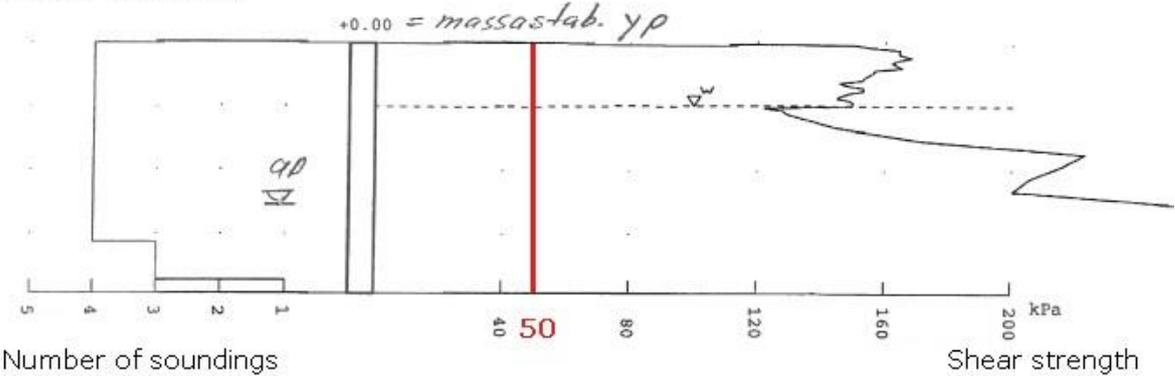
Figure 1.6a. The average shear strength of stabilised peat in block 3 VPL-4. The age of the mass stabilisation is 87 days. The used binder material mixture is EF PF + KS 180 + 100 kg/m<sup>3</sup>.
