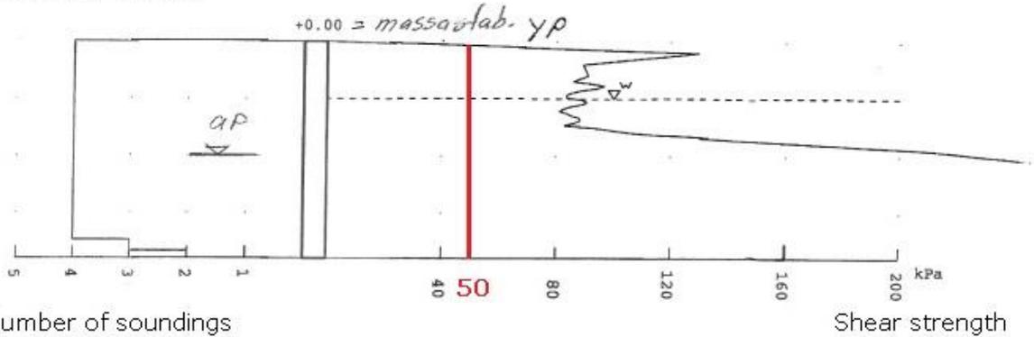
Figure 1.8a. The average shear strength of the stabilised peat in block 1 VPL-5. The age of the mass stabilisation is 67 days. The used binder material mixture is EF CFB + KS 200 + 80 kg/m<sup>3</sup>.
