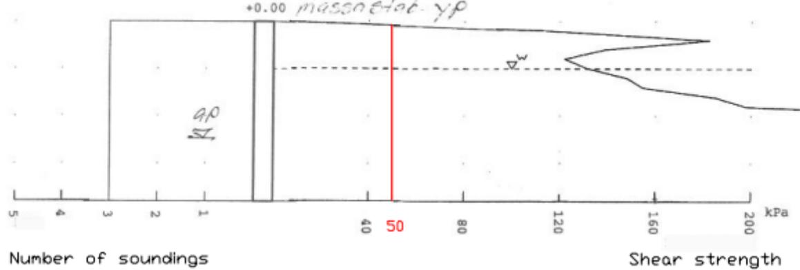
Figure 1.5b. The average shear strength in block 11 VPL-3 at the age of ten months.
