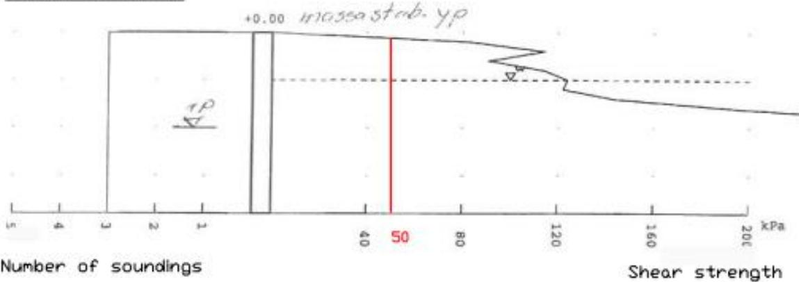
Figure 1.8b. The average shear strength in block 2 VPL-5 at the age of ten months.
