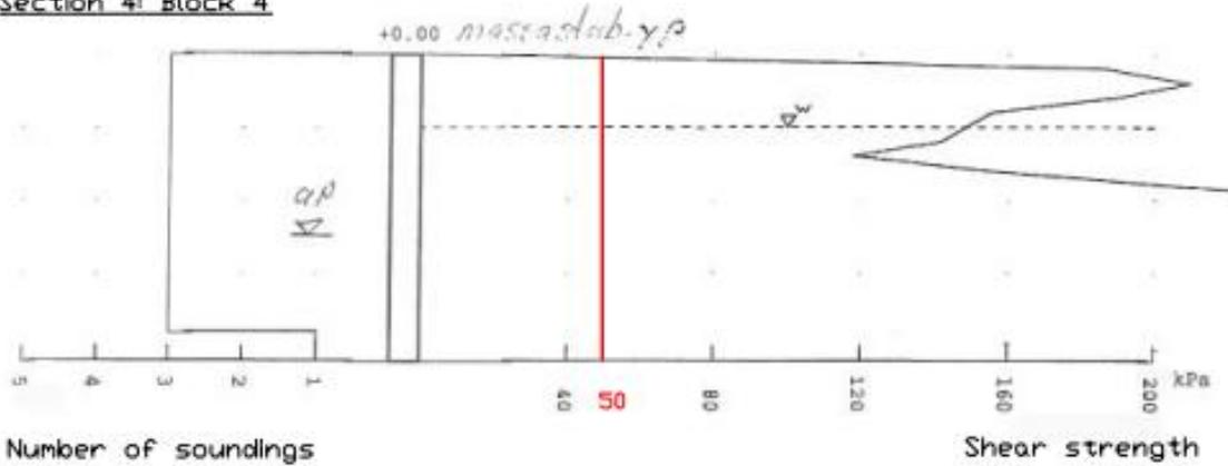
**Figure 1.6b. The average shear strength in block 4 VPL-4 at the age of ten months.**
