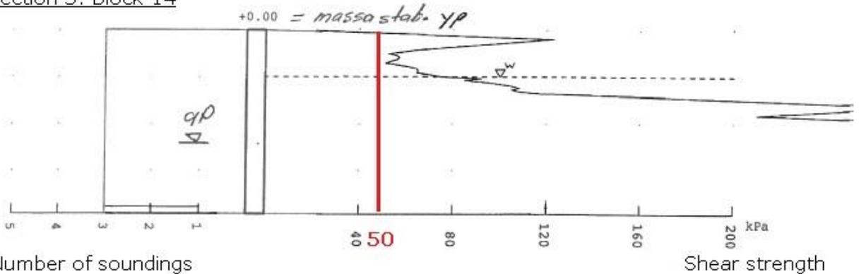
Figure 1.9. The average shear strength of the stabilised peat in block 14 VPL-5. The age of the mass stabilisation is 85 days. The used binder material mixture is EF CFB + KS 200 + 80 kg/m<sup>3</sup>.
