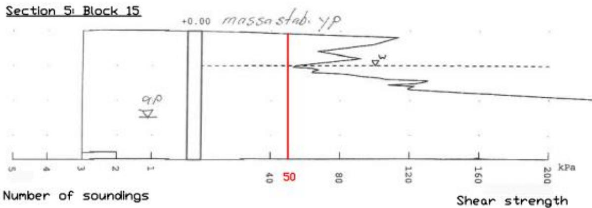
**Figure 1.9b. The average shear strength in block 15 VPL-5 at the age of ten months.**
