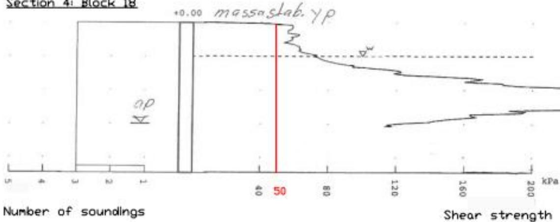
**Figure 1.7b. The average shear strength in block 18 PPL-4 at the age of ten months.**
