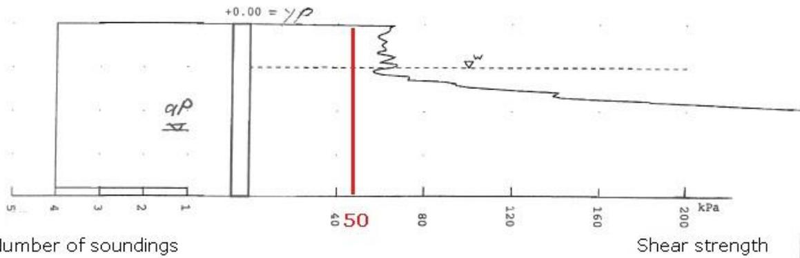
Figure 1.5a. The average shear strength of stabilised peat in block 12 VPL-3. The age of the mass stabilisation is 76 days. The used binder material mixture is EF PF + KS 170 + 110 kg/m<sup>3</sup>.
