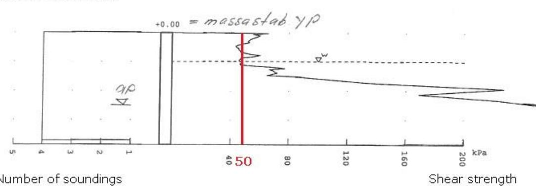
**Figure 1.4a.** The average shear strength of stabilised peat in block 11 VPL-2. The age of mass stabilisation is 104 days. The used binder material mixture is EF PF + KS 190 + 90 kg/m<sup>3</sup>.
