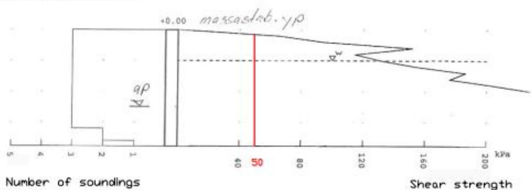
**Figure 1.4b.** The average shear strength in block 10 VPL-2 at the age of ten months.
