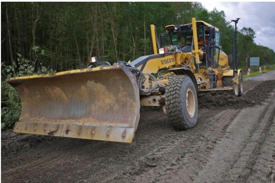
**Figure 4-7. Road grader shaping freshly mixed road base**
