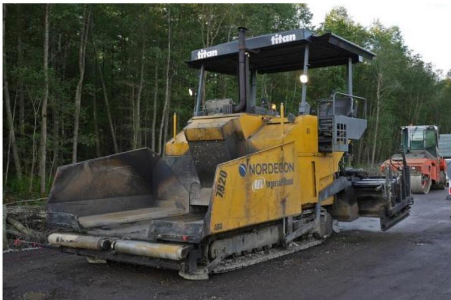
Figure 4-3. Asphalt paver used for wet binding agent mixture spreading
