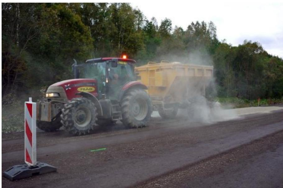
**Figure 4-9. Tractor-pulled cement spreading car**
