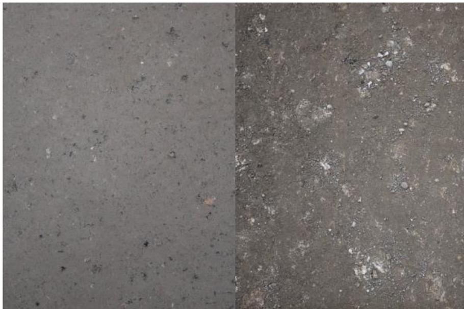
**Figure 4-11. Left: surface of the „too wet section”, right: surface of the „drier section”**
