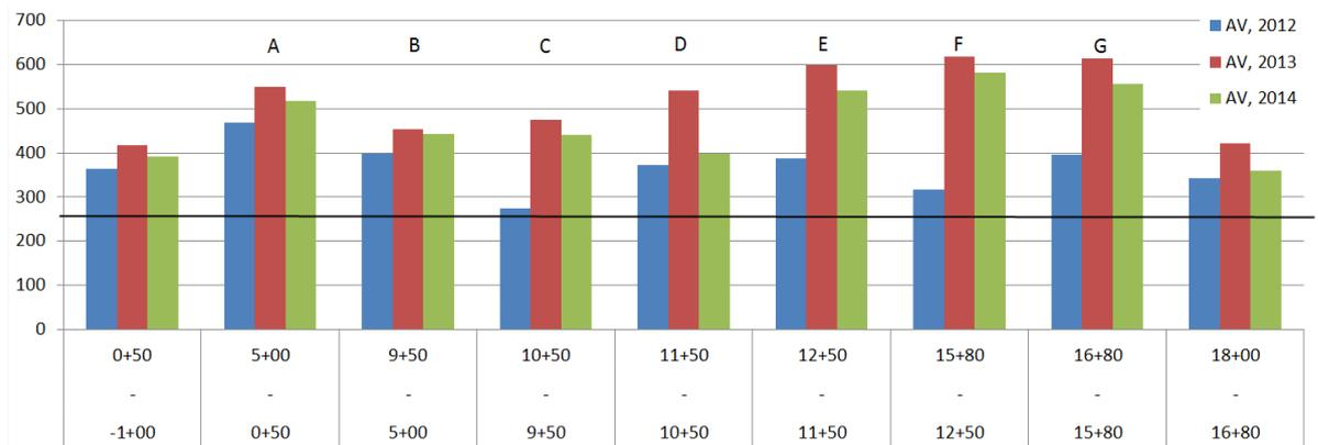
**Figure 6-3. Progress of bearing capacity (comparison of FWD results 2012-2014)**
