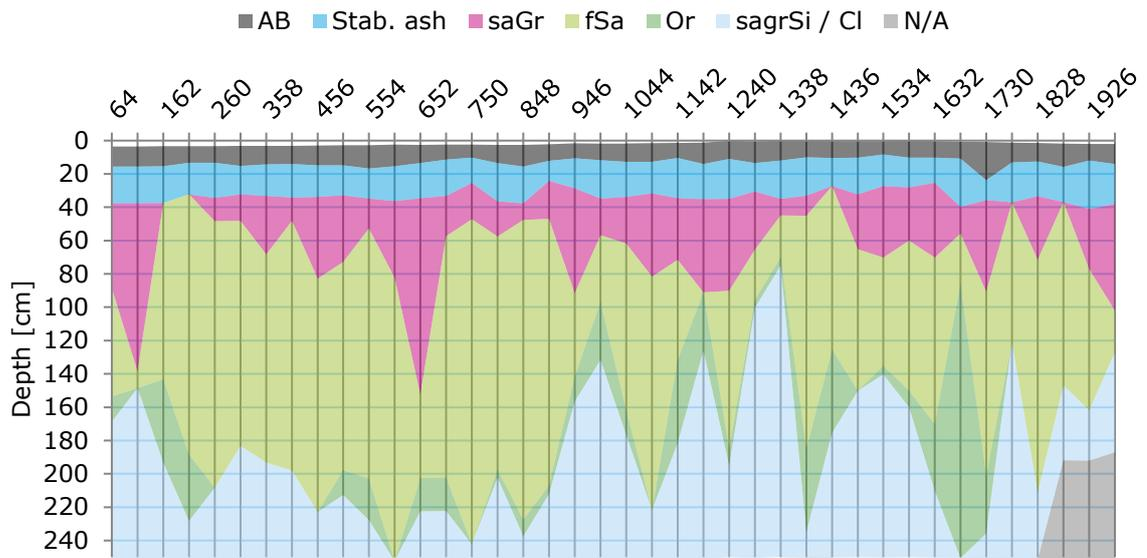
**Figure 2-3. Longitudinal structure of the section before repairs. Horizontal: distance from STA 0 (located in the 16.1 km mark of road 13109)**
