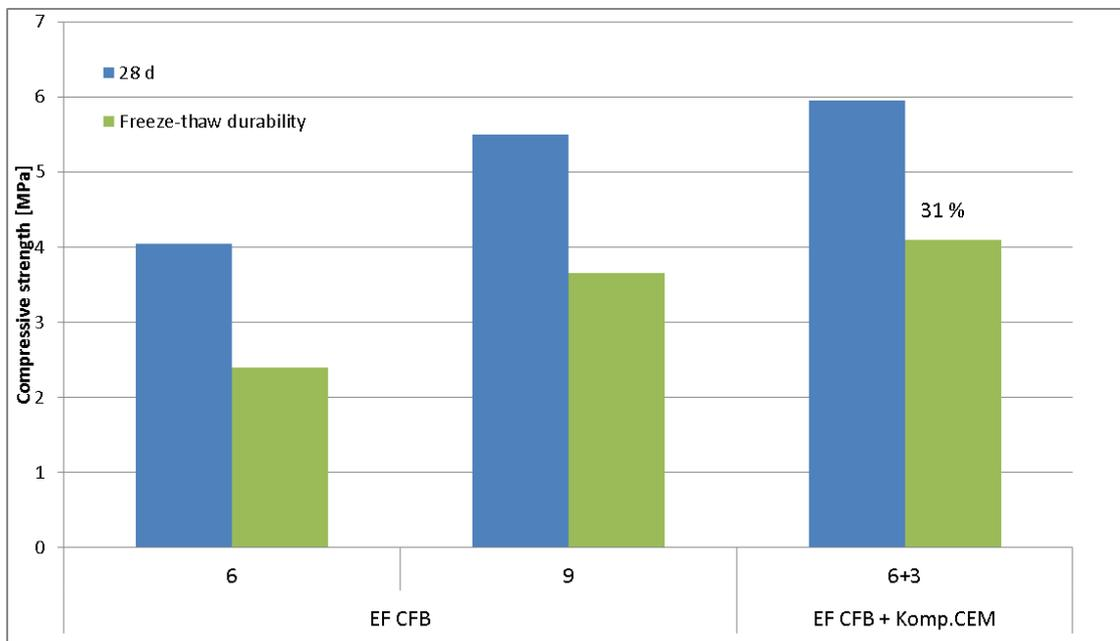
Figure 3-4. Stabilisation test results for Aidu mining waste (aggregate)
