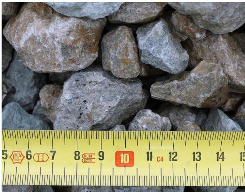
Figure 3-7. Aidu 16-32 mm aggregate
