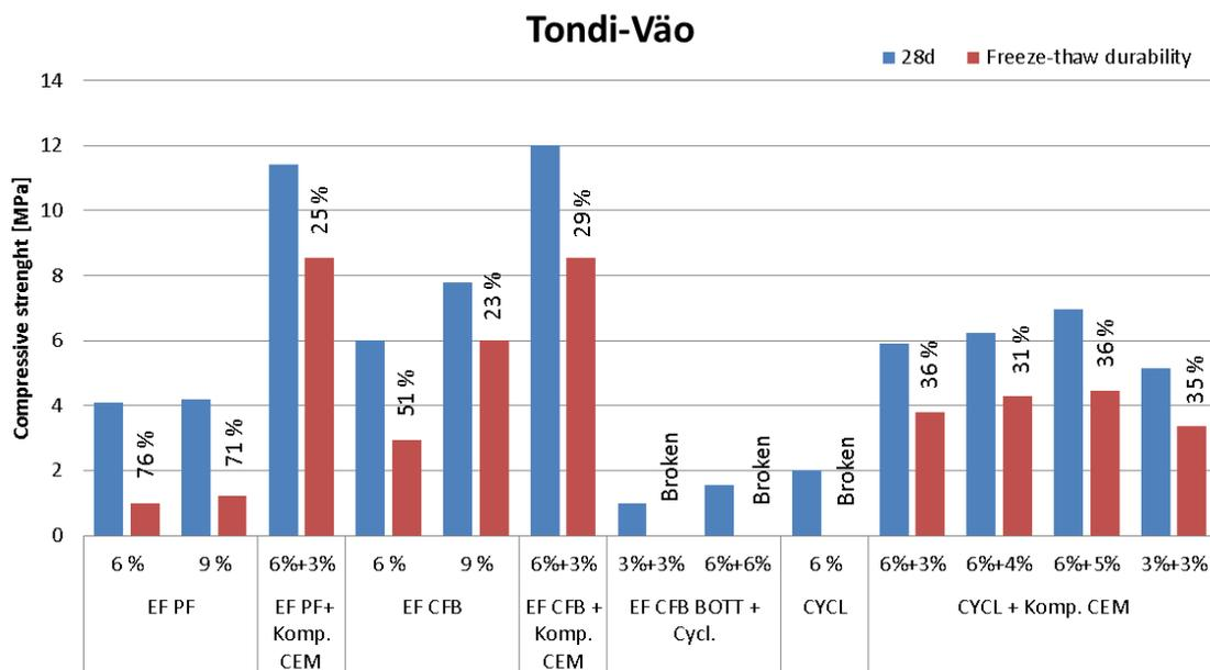
**Figure 3-2. Stabilisation test results for Tondi-Väo aggregate**
