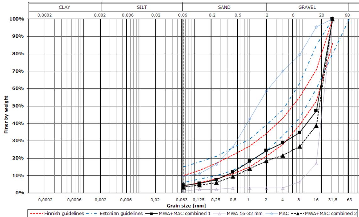
Figure 3-6. Grading curve (Est and Fin guidelines and estimates for MWA and MAC).
