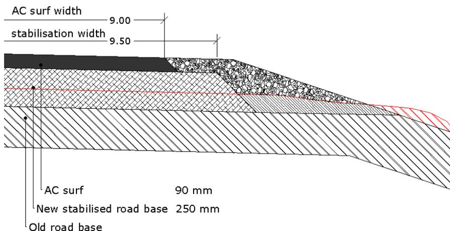
**Figure 3-9. Extract of Cross section (STA 0+50-9+50). Red line - old road structure**
