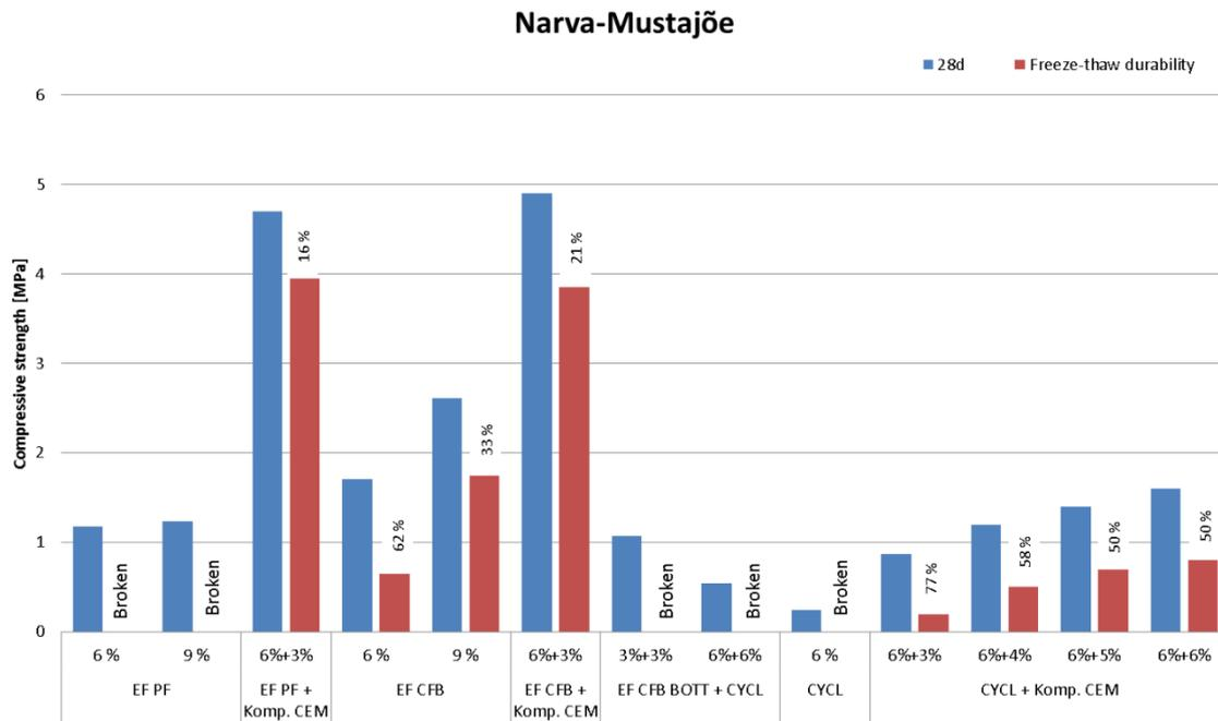
**Figure 3-5. Stabilisation test results of Narva-Mustajõe road material**
