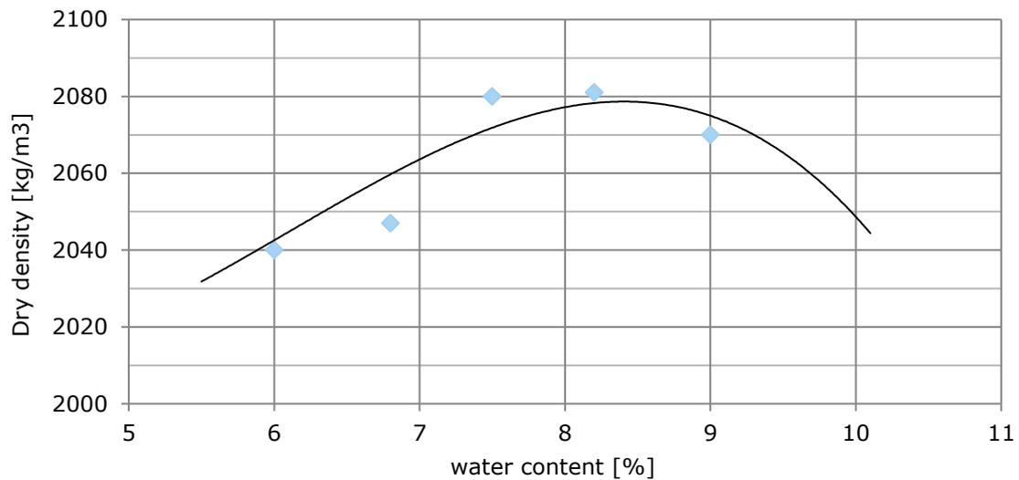
**Figure 4-16. Mod. Proctor compaction results (STA 5+20). Binder: 5% OSA CYCL. + 5% KC**
